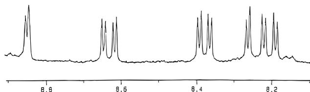
**Figure 1.**  $^1\text{H}$  NMR for the pyrrole of  $\text{Rh}(\text{CH}_2)_6\text{Rh}(\mu\text{-C}(\text{O})\text{C}(\text{O}))$  (**2**) in  $\text{C}_6\text{D}_6$  (296 K).
