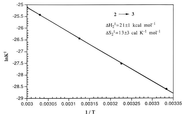
**Figure 2.** Determination of the activation parameters for the dissociation of  $\text{Rh}(\text{CH}_2)_6\text{Rh}(\mu\text{-C}(\text{O})\text{C}(\text{O}))$  (**2**) into  $[\text{OCRh}(\text{CH}_2)_6\text{RhCO}]^{\cdot}$  (**3**) using proton NMR line broadening of **2** as the observable ( $k_f = \tau_d^{-1}$ ;  $K^{\ddagger} = k_f(h/kT)$ ).
